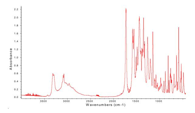
Fig. 40 IR spectrum of thifensulfuron-methyl standard
